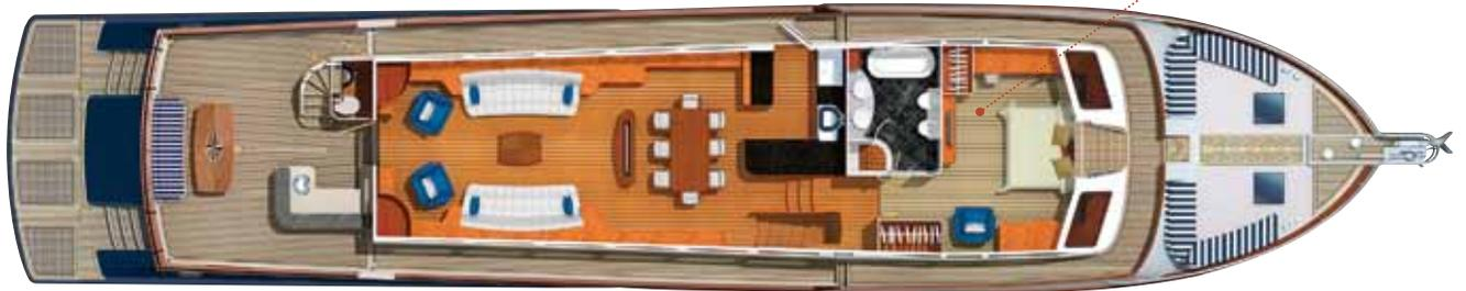
**AFT DECK:** An hydraulic transom door and swim platform host water toys and secondary access to the crew area and engine room.
